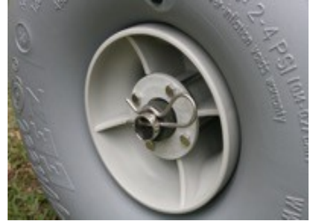
Reinstall Hitch Pin to retain wheels.
