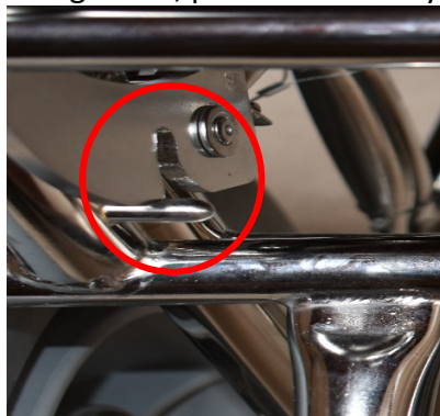
Locking bar and pin disengaged.
