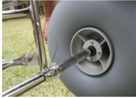
Install wheel onto axle.
