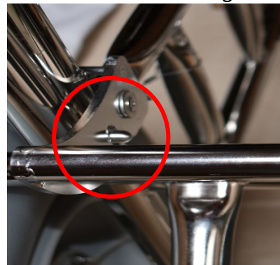
Locking bar and pin engaged.
